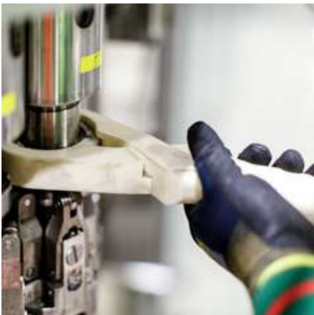
This ergonomically optimized tool works by interfacing with a 3D printed collar
