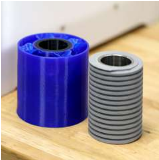
Operators can adjust dampening levels by changing the infill percentage of the 3D printed part (on the left)
