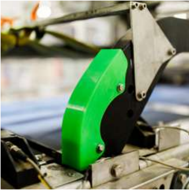
This simple part reduces the risk of snagging hair or clothing in the chain
