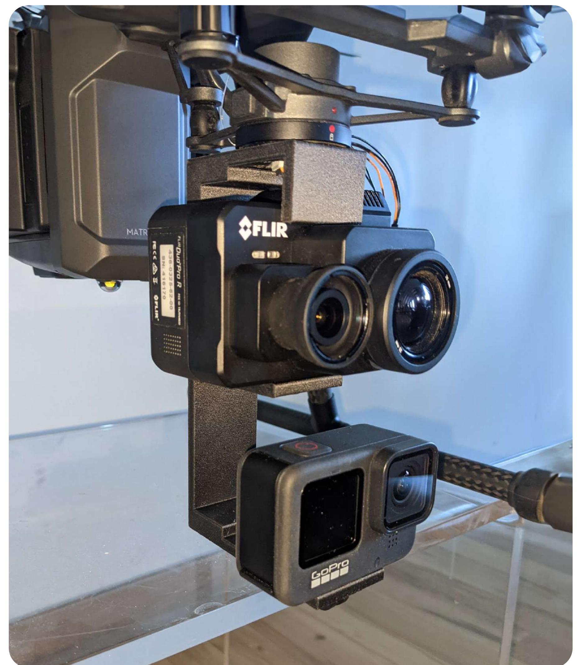
Part of the Dragontech platform incorporates the LIDAR, Multi-Spectral Spectral Sensors, and a controller attached to an enterprise drone via mounts 3D printed on the MakerBot METHOD X using Nylon Carbon Fiber.
