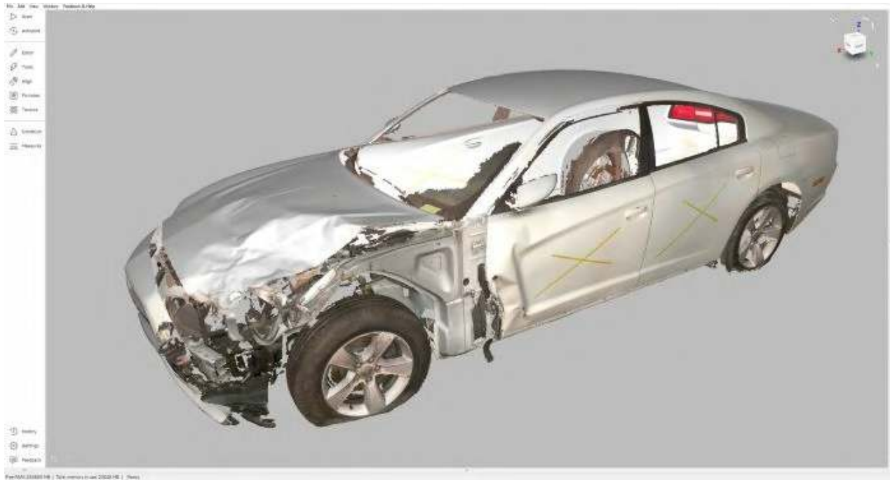
Artec Studio software screenshot showing the Leo scan of the 2014 Dodge Charger
