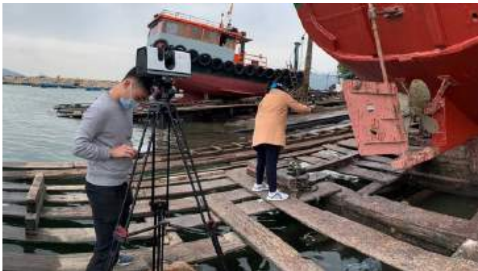
Artec Ray is used for capturing boats, ships, and surfaces that may have led to the animal's injury or death
