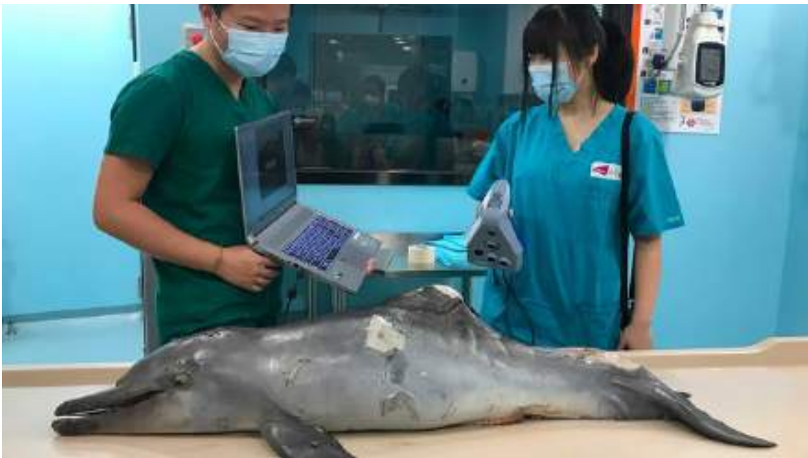
A dolphin being scanned with Artec Space Spider
