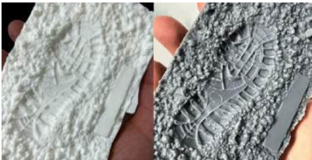
3D-printed scale models of forensic footwear impressions, for demonstration purposes. Photo: Eugene Liscio, P.Eng., ai2-3D Forensics
