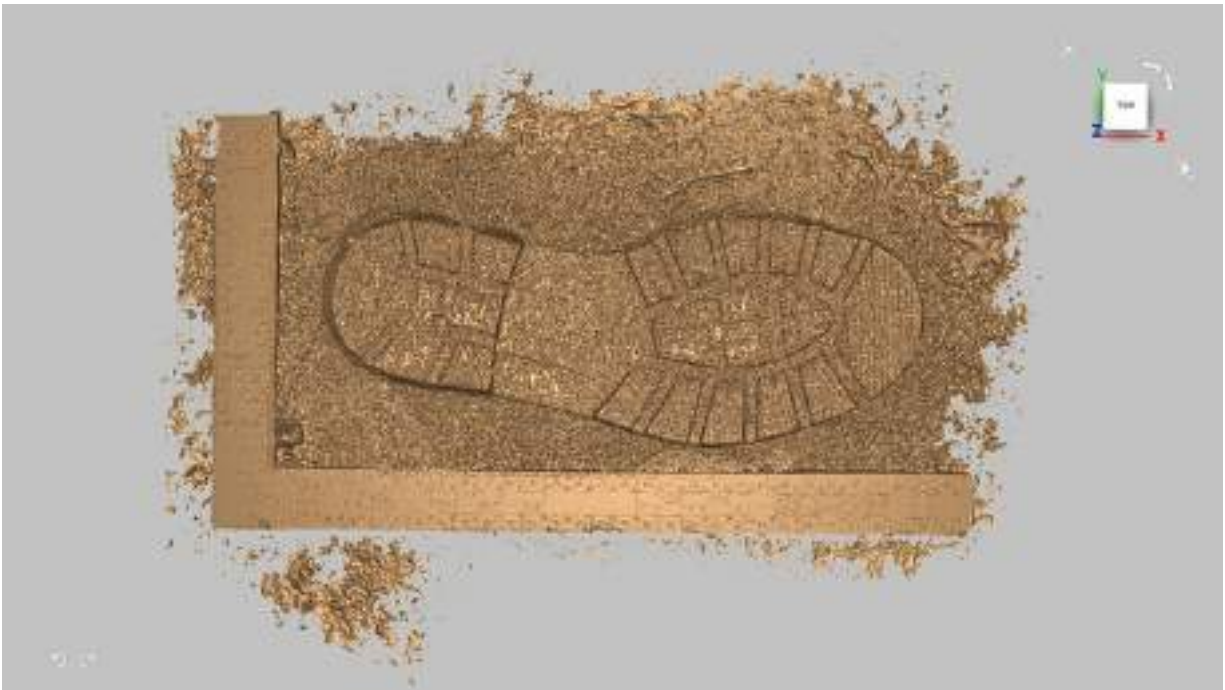
Artec Studio screenshot showing Space Spider scan of a boot impression. Photo: Eugene Liscio, P.Eng., ai2-3D Forensics
