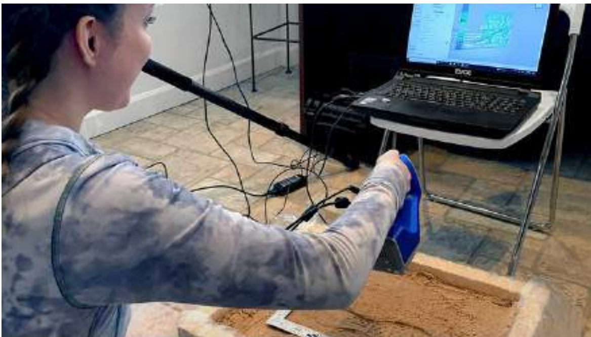
Watching the 3D evidence come to life: forensic science researcher Julia Harvey documenting a 3D footwear impression with the Artec Space Spider. Photo: Eugene Liscio, P.Eng., ai2-3D Forensics
