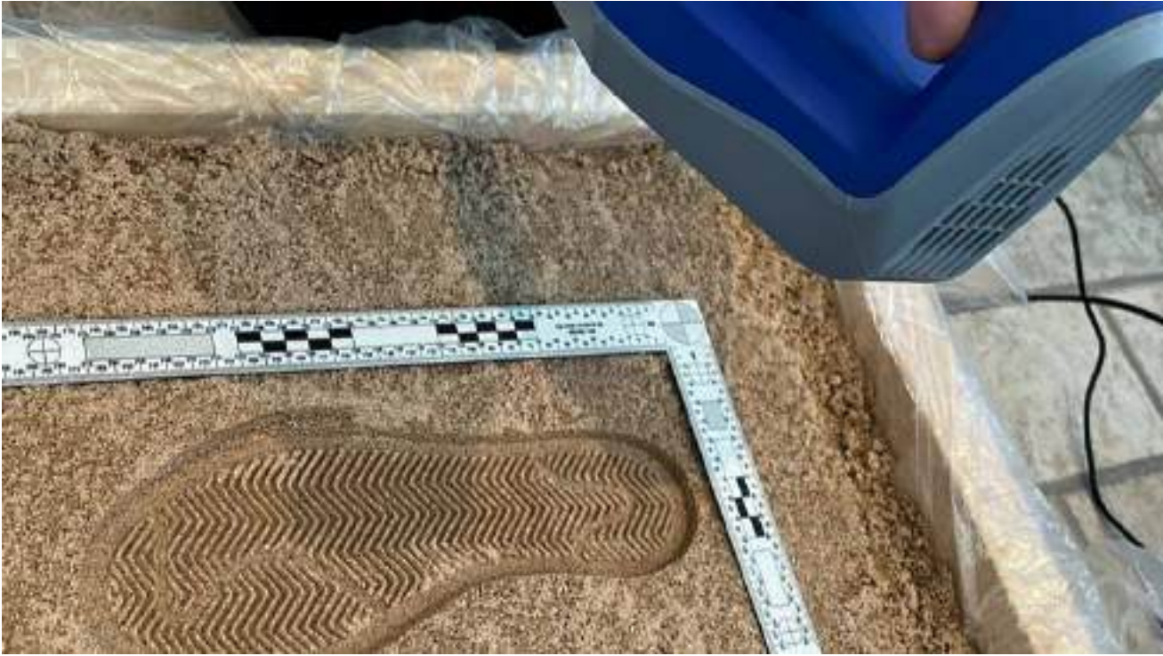
Forensic science researcher Julia Harvey using the Artec Space Spider to document a 3D footwear impression. Photo: Eugene Liscio, P.Eng., ai2-3D Forensics
