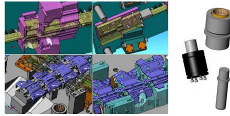
No die design software is complete unless it has a thorough **Intelligent** Standard Component Library. The Logopress3<sup>™</sup> library not only inserts the component you select but also cuts every hole in each plate and automatically manages all mates.
